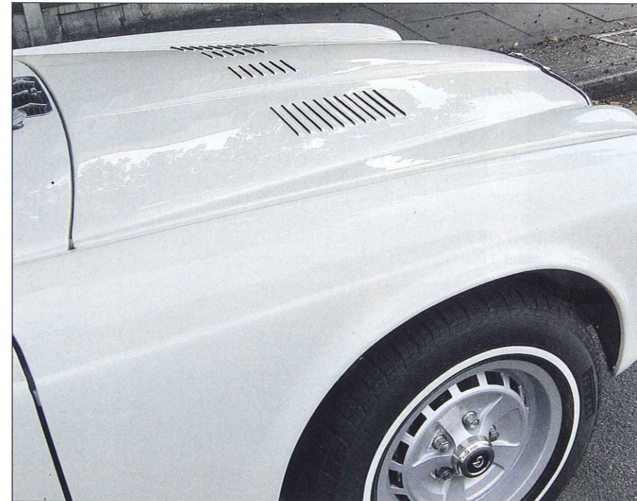
Mark likes the lowers and they help keep the engine cool.
