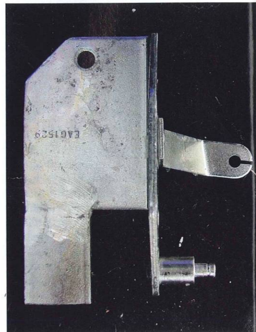
The accelerator bracket which the rotating spindle mounts on to. Note this has had a new piece of metal welded at the bottom which is drilled with 2 x 10mm holes to move it down level with the HD8 carb linkages. This was a spare unit welded and zinc plated.
